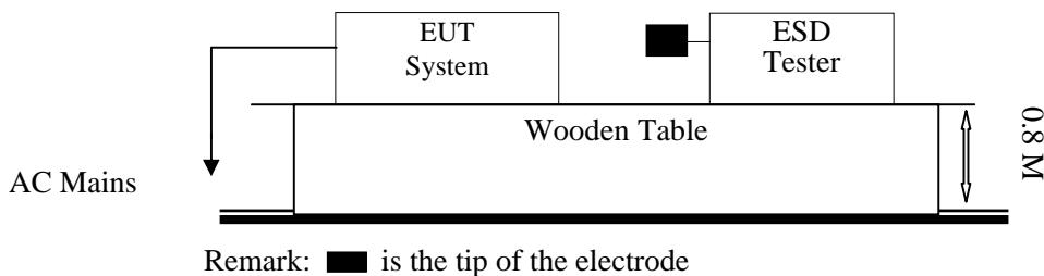
EN 61000-4-2 specifies that a tabletop EUT shall be placed on a non-conducting table which is 80 centimeters above a ground reference plane and that floor mounted equipment shall be placed on a insulating support approximately 10 centimeters above a ground plane. During the tests, the EUT is positioned over a ground reference plane in conformance with this requirement.
