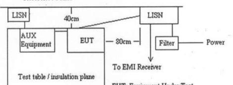
EUT: Equipment Under Test LISN: Line Impedence Stabilization Network
