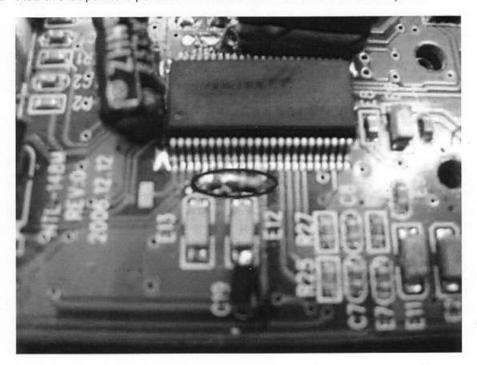
3. Replace the Capacitor E3 and E5 with new ones which are 100µF/10V.
